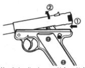
Move the barrel/receiver assembly forward to free it from the internal hook at the front of the frame.
