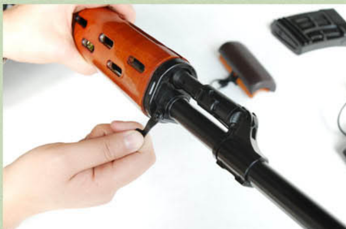
Rotate the handguard catch button 180° clockwise
