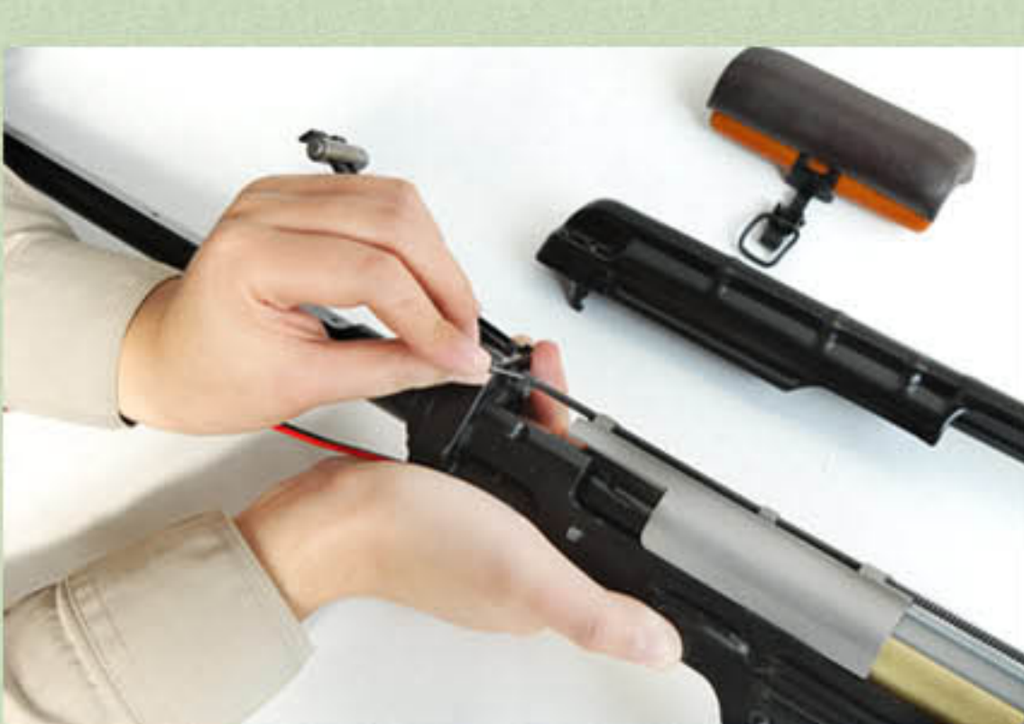
Loosen the adapter of holding lever by hexagon wrench.
