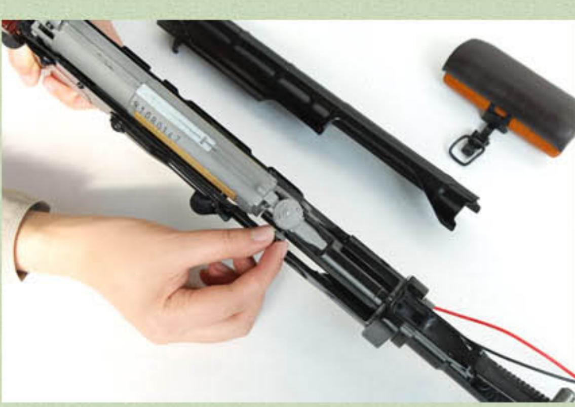
Loosen the hop-up fixed screws anticlockwise, and then take them down.
