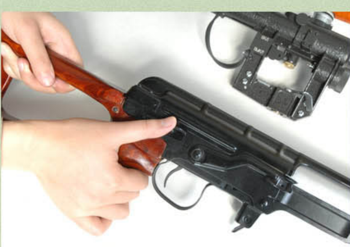
Move the receiver cover pin clockwise to backstop point.
