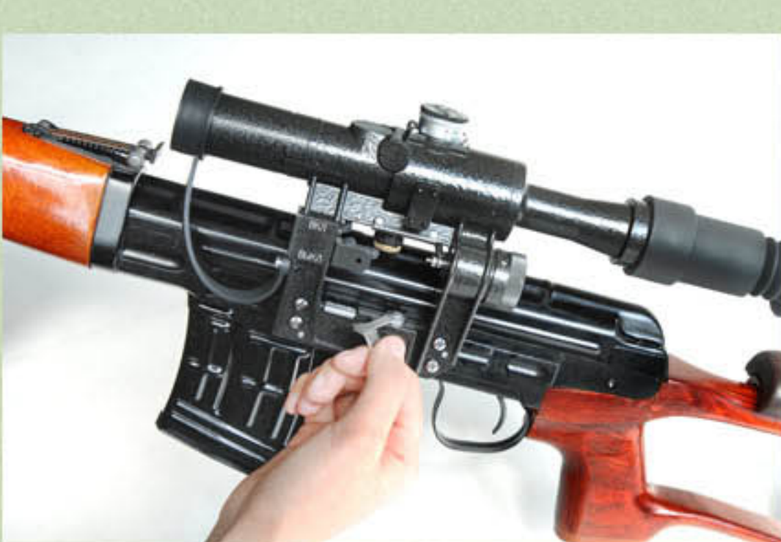
Open the scope release latch backward, and then take down the scope.
