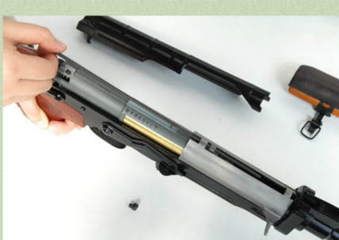
Pull it backward, remove holding lever and spring, and then take down the cocking lever.
