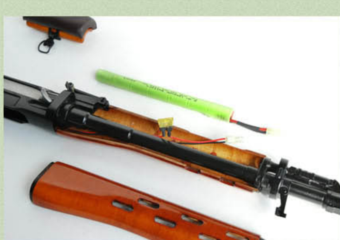
Take down the left and right handguard, and take out the battery
