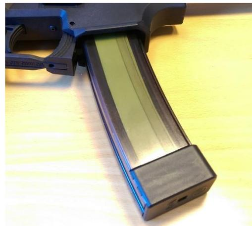
4. Slide your design into the magazine as shown. Replace pin and bottom cap to finish the job.
