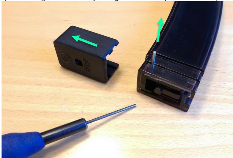
**NOTE** the magazine inner part is no longer locked and can be pushed out which is not necessary to do in order for you to mount your design – If you do anyway – beware of the springs!
