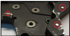
Fig. 6 - To fit cables into the gear-box, grind pins in red circles
